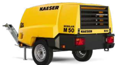
COMPRESOR PORTÁTIL KAESER M50 185 cfm
