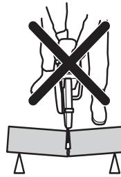
If the cutting equipment is pinched or stalled in the kickback zone, the reactive force will push the machine up and back towards the user in a rotating motion causing serious or even fatal injury.
